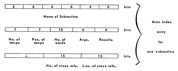
The first word of the entry consists of the name of the subroutine in six six-bit excess-three characters.
